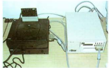
Cross Products' development system works with SOA's CartDev box (left) and also the company's new Mirage CD emulator (right)
